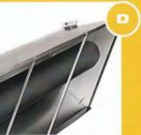
Focus Shield Reflectors and Closed Reflector Ends extend below tube surface to trap convection heat and convert it to useable infra-red heat. Provides additional comfort and fuel savings.
